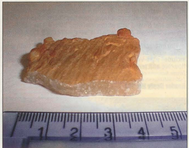
Electronic water conditioning can cause encrusted scale to break away in large lumps, for easy removal by manual cleaning.
