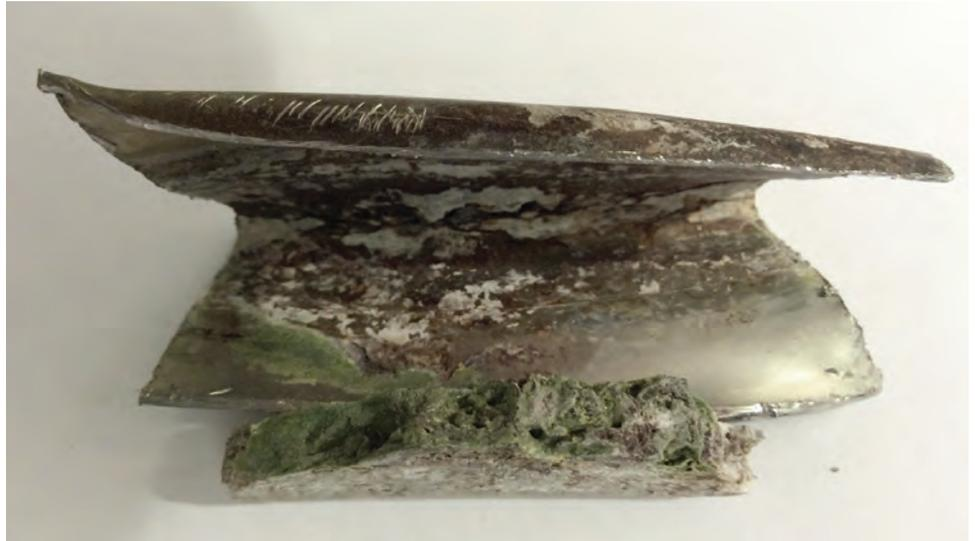
An example of debris scale that has accumulated in a Geononi heat exchanger causing it to fail
